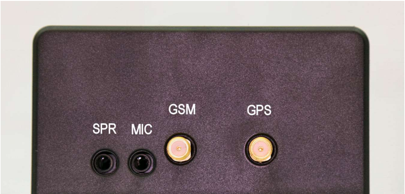
Here is a close-up of the audio and antenna ports on the side of the enclosure. The Speaker and Mic ports are reserved for future expansion and are not currently in use. There is also a connector for a GSM (cellular) and GPS antenna.
